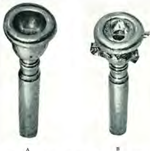
FIG. 51.—Mouthpiece of cornet. A, Rim is not detachable. B, During construction of replica of mouthpiece rim (see text).
